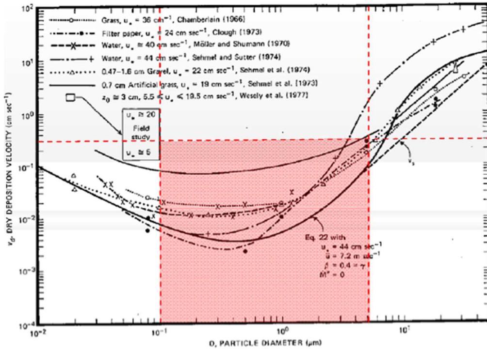
Fig. 4 Dry deposition velocity as a function of particle size. Data were obtained from a number of publications.<sup>19-25</sup> The theoretical curve appropriate for a smooth surface is shown for comparison. Note that the theoretical curve is strongly dependent on the value for  $u_*$  and that Eq. 22 does not contain a parameterization for surface roughness. For a preliminary study of the effect of surface roughness and other factors, see Ref. 5.
