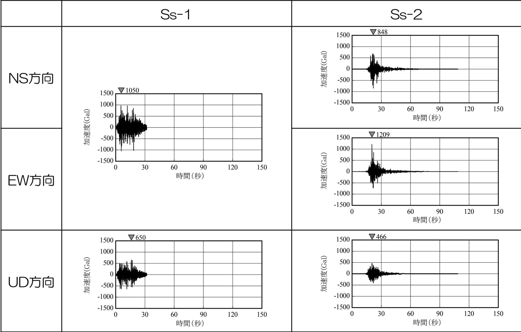
大湊側 入力地震動（基準地震動S<sub>s</sub>）時刻歴波形(2)
