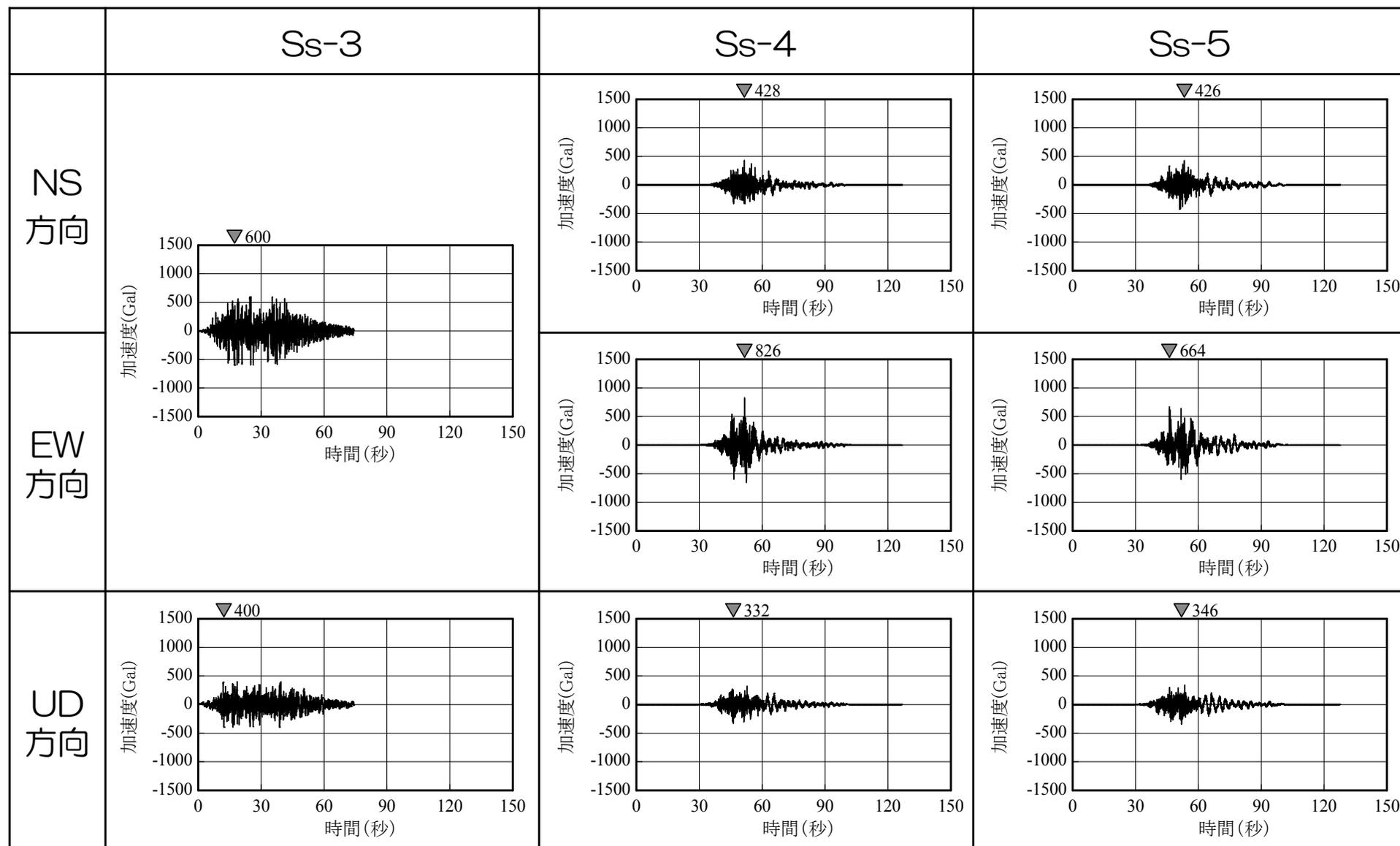
大湊側 入力地震動（基準地震動S<sub>s</sub>）時刻歴波形(3)
