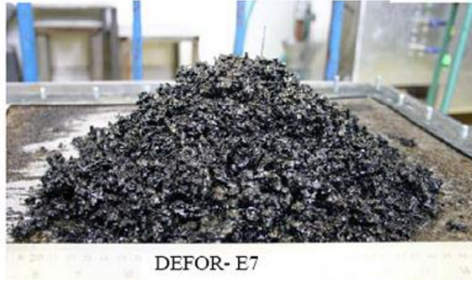
図付 3-6 DEFOR-E 実験後のデブリ状態 [16]
