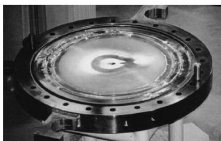
Inlet of test piece (White powder is CsI aerosol)
