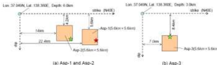
Figure 2 Source model of the Niigataken Chuetsu-oki earthquake ( M=6.8 ). The red star and green stars indicate the location of the epicenter (the rupture start point of Asp-1) and the rupture start points of Asp-2 and Asp-3, respectively.
