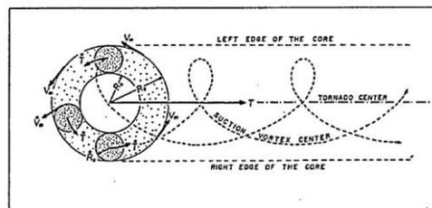
Figure 8.2 Fujita's latest model of multiple-vortex tornadoes for engineering applications. The design-basis tornado model in Chapter 6 developed in 1977 was identified as "DBT-77". Design-basis suction-vortex parameters in Chapter 7 were added to the DBT-77 in constructing this latest analytical model, to be identified as "DBT-78".
