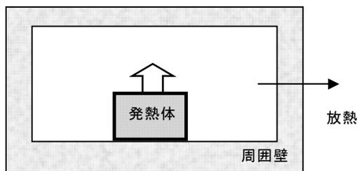
$$TR' = TR + \frac{t \times (q - qi)}{60 \times (\text{室内の熱容量})}$$
