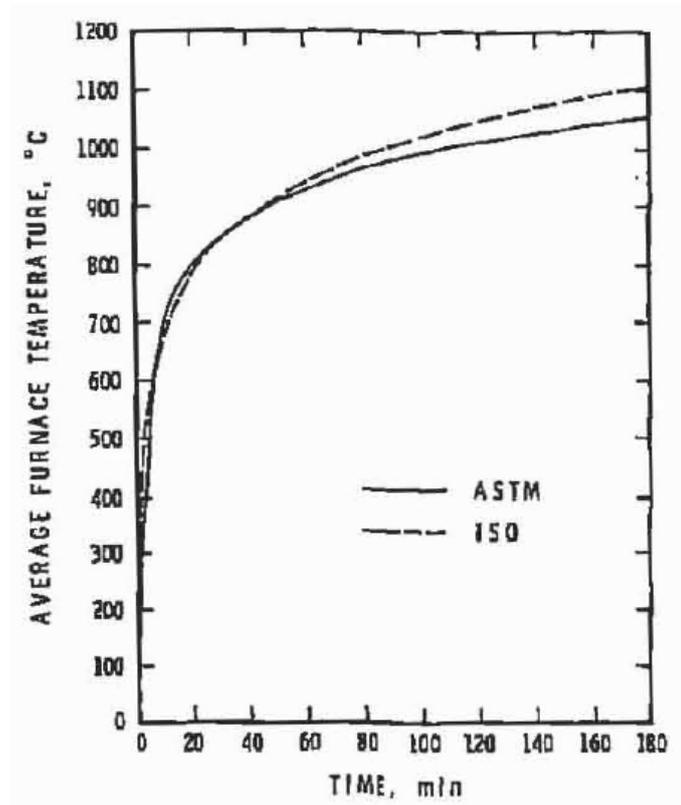
第 11 図 加熱曲線の比較(出典:Comparison of Severity of Exposure in ASTM E119 and IS0834 Fire Resistance Tests)
