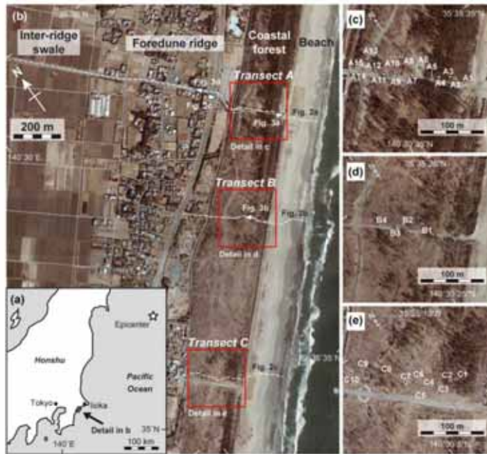
Fig. 1 Locations of the Hasuruma site and the surveyed transects. (a) Index map of eastern Japan showing the position of the Hasuruma site and the epicenter of the 2011 Tohoku-oki earthquake (star). (b) Aerial view of the Hasuruma site showing the major geomorphic features, topographic survey lines (dashed lines), and the locations of the views shown in panels c-e (rectangles), and of the photographs shown in Fig. 3 (arrows). (c) Survey locations along transect A. Pencil samples were acquired at locations marked by filled circles. (d) Survey locations along transect B. (e) Survey locations along transect C. Aerial photos in panels b-e are from the Geospatial Information Authority of Japan (DXF-2011-4-C2F-1, 2, 3) and were taken in February 2012.
