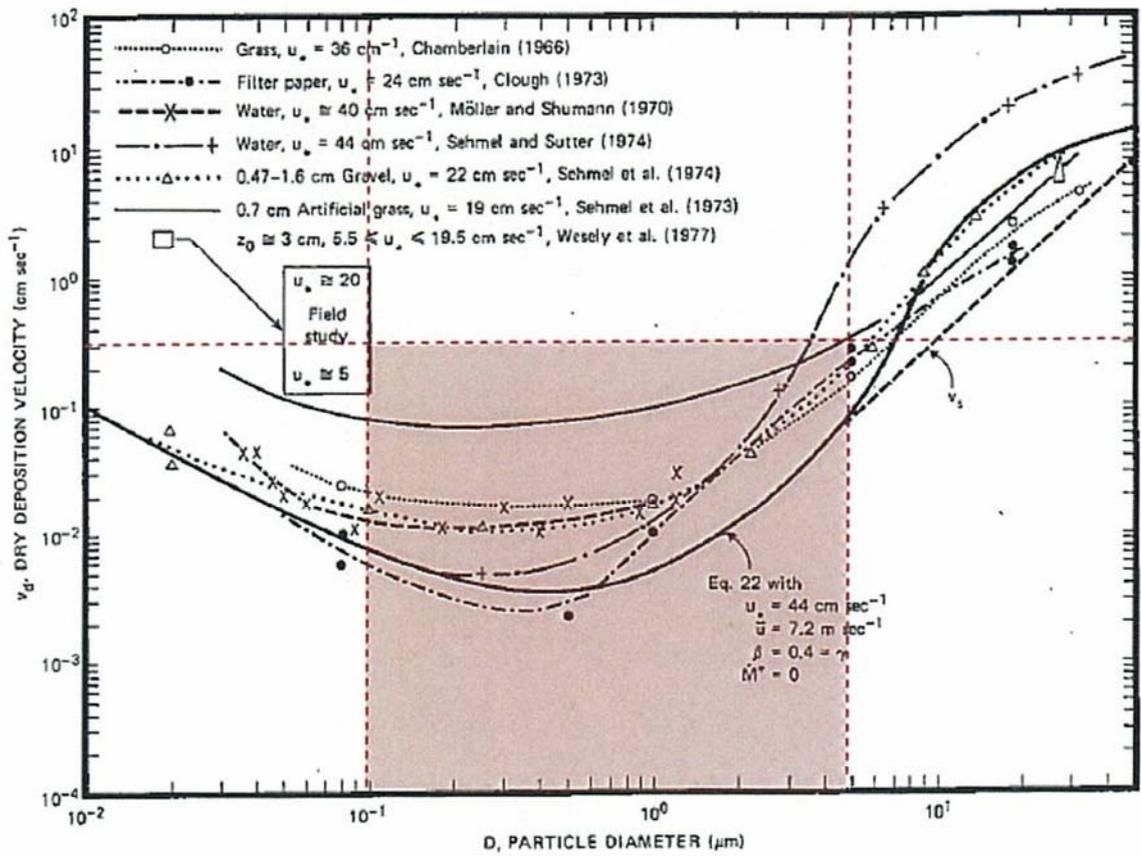
Fig. 4 Dry deposition velocity as a function of particle size. Data were obtained from a number of publications.<sup>1,9-23</sup> The theoretical curve appropriate for a smooth surface is shown for comparison. Note that the theoretical curve is strongly dependent on the value for  $u_*$  and that Eq. 22 does not contain a parameterization for surface roughness. For a preliminary study of the effect of surface roughness and other factors, see Ref. 5.
