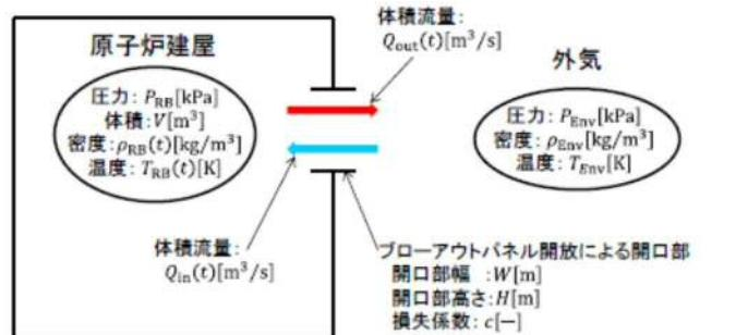
$$\rho_{RB}(t) V C_{P\_RB} \frac{dT_{RB}(t)}{dt} = \rho_{Env} n Q_{in}(t) C_{P\_Env} T_{Env} - \rho_{RB} n Q_{out}(t) C_{P_{RB}} T_{RB}(t)$$
