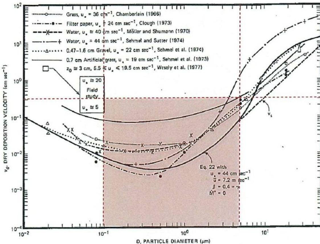
Fig. 4 Dry deposition velocity as a function of particle size. Data were obtained from a number of publications.<sup>19-25</sup> The theoretical curve appropriate for a smooth surface is shown for comparison. Note that the theoretical curve is strongly dependent on the value for  $u_*$  and that Eq. 22 does not contain a parameterization for surface roughness. For a preliminary study of the effect of surface roughness and other factors, see Ref. 5.
